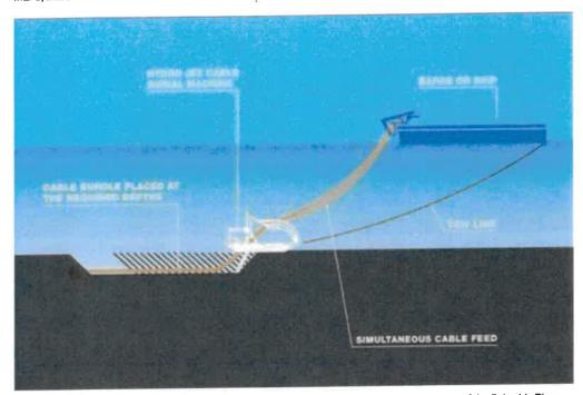
A barge or ship and towed submarine system will be used to lay a power under sediment at the bottom of the Columbia River between The Dalles and Vancouver.
